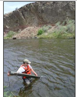
Deployment of water chemistry monitoring instrument in the John Day River, June 2010
