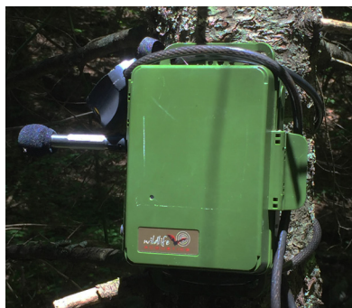
An acoustic detector attached to a tree. NPS photo.
