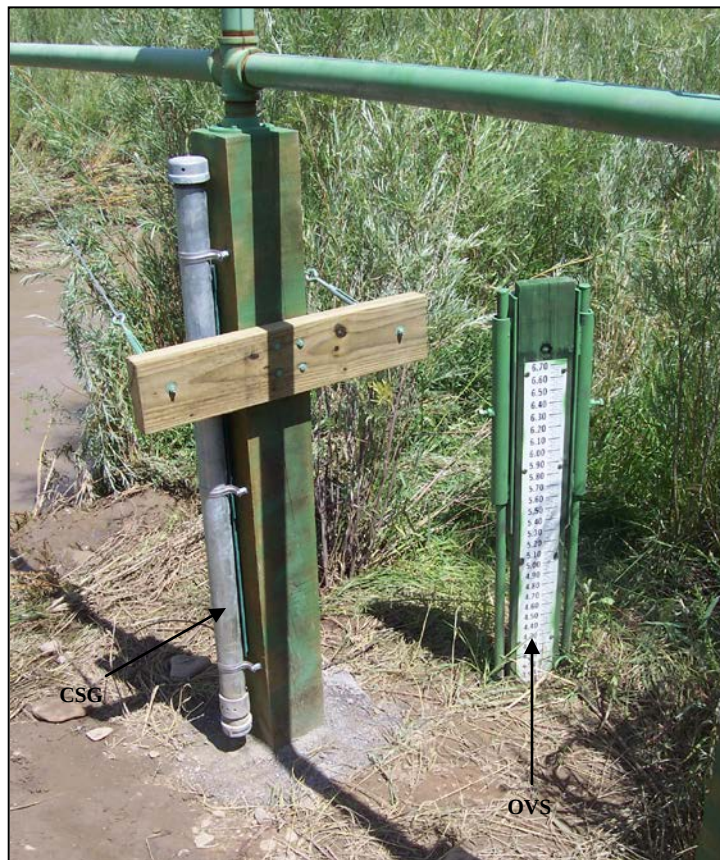
Figure 11: Crest-stage-gage (CSG) and high stage vertical staff (OVS 2) at Mancos River at Anitas Flat Station. Photograph taken August 15, 2005 by Gwen Gerber.
