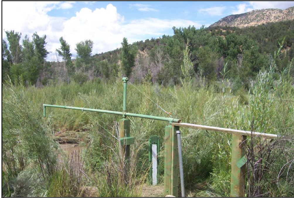
Figure 10: Cantilever (OHS) at Mancos River at Anitas Flat Station. Photograph taken August 15, 2005 by Gwen Gerber.
