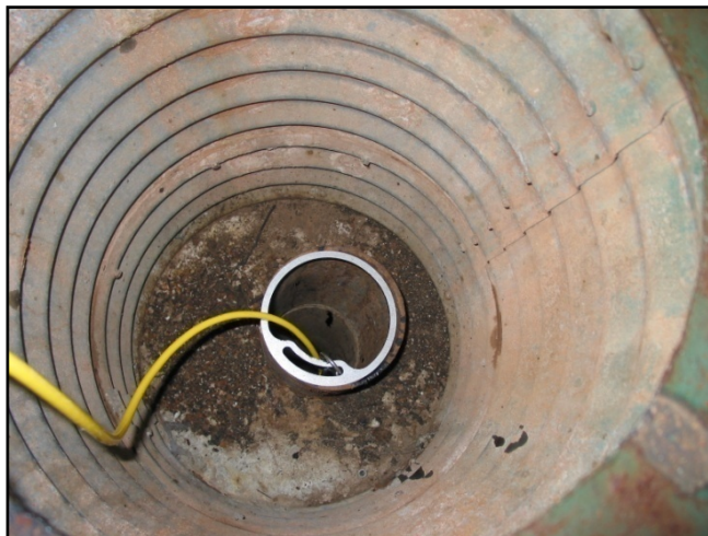
FIGURE 5: East Observation Well, well dock and carabineer within well casing.
