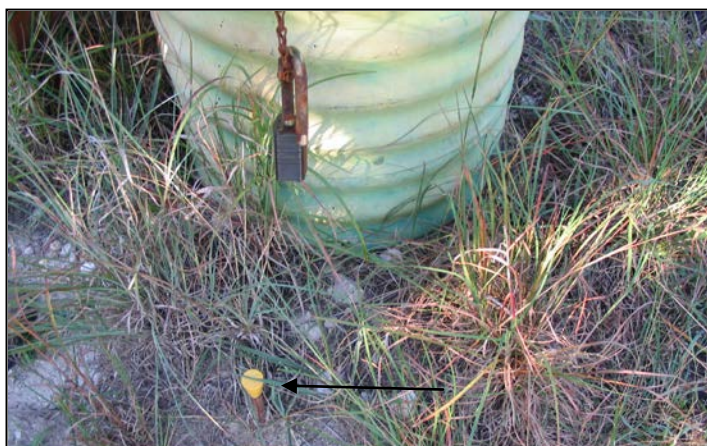
FIGURE 10: Reference Mark 1 (RM1) 1/2 inch rebar with yellow cap, centered in front of corrugated housing
