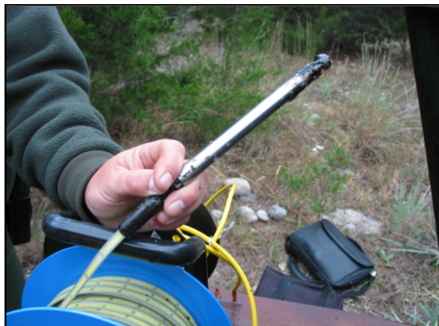
FIGURE 8: Electric tape covered in tar.
