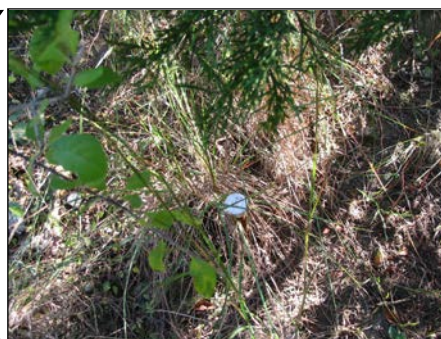
FIGURE 9: Reference Mark 2 (RM2) 1/2 inch rebar with aluminum cap.
