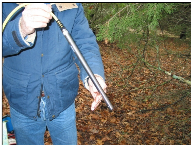
FIGURE 4: Design Analysis Associates Inc. WaterLog DH-21 0-15 PSI submersible pressure/temperature transducer/data logger (Design Analysis Associates, Inc. 2010a).
