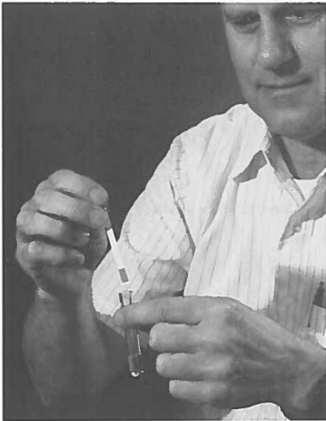
Figure 1. Inserting litmus paper stick into test tube of meltwater.
