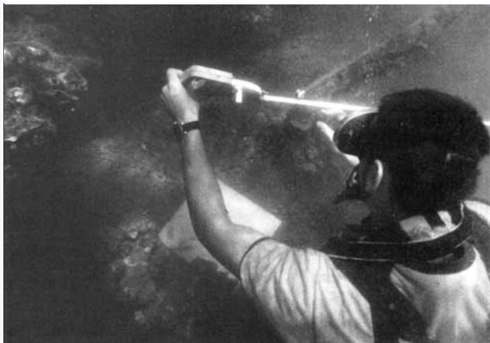
Figure 3.3. After being drawn, each feature is measured back to two points on the baseline. This allows accurate mapping through a simple geometric procedure called trilateration. (NPS photo by Larry Murphy)
