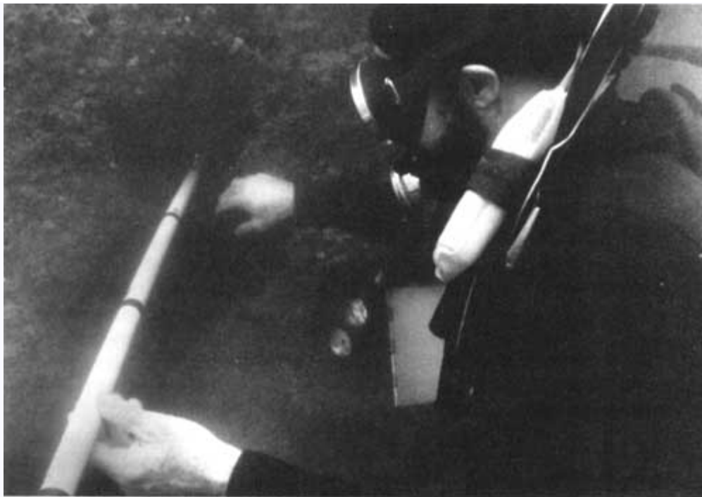
Figure 4.10. Water is drawn from interior spaces of the USS ARIZONA to surface through a PVC pipe and vinyl tube. Pipe is marked to establish exact distance of penetration. (NPS photo by Larry Murphy)
