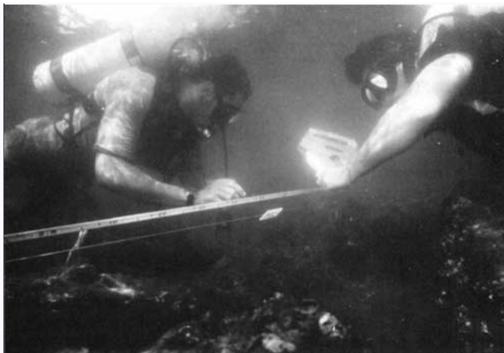
Figure 3.1. U.S. Navy divers add marked clips every 10 feet to survey line on USS ARIZONA after it was installed by NPS underwater archeologists. (NPS photo by Larry Murphy)
