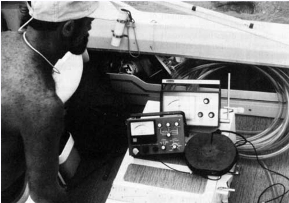
Figure 4.11. On the surface, water drawn from inside the wreck was analyzed for oxygen, temperature and pH levels. (NPS photo by Larry Murphy)
