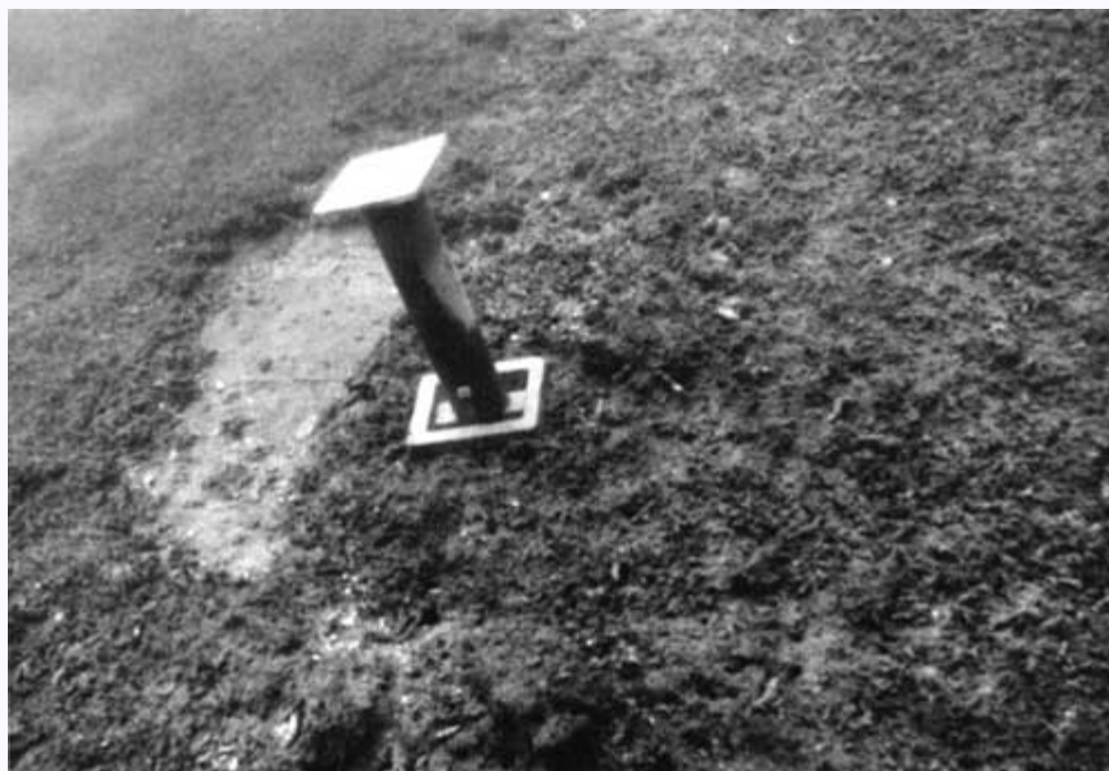
Figure 4.7B. Horizontal surface monitoring station marker in place. (NPS photo by Larry Murphy)
