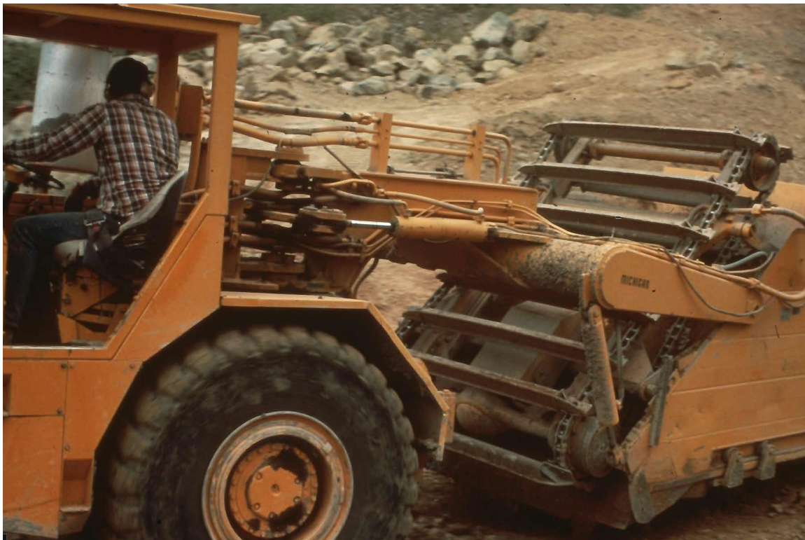
Unit: 86-4 Date: 8-26-86, M-6-1 Michigan 110-110B Elevating Scraper, 50mm, (GB)
