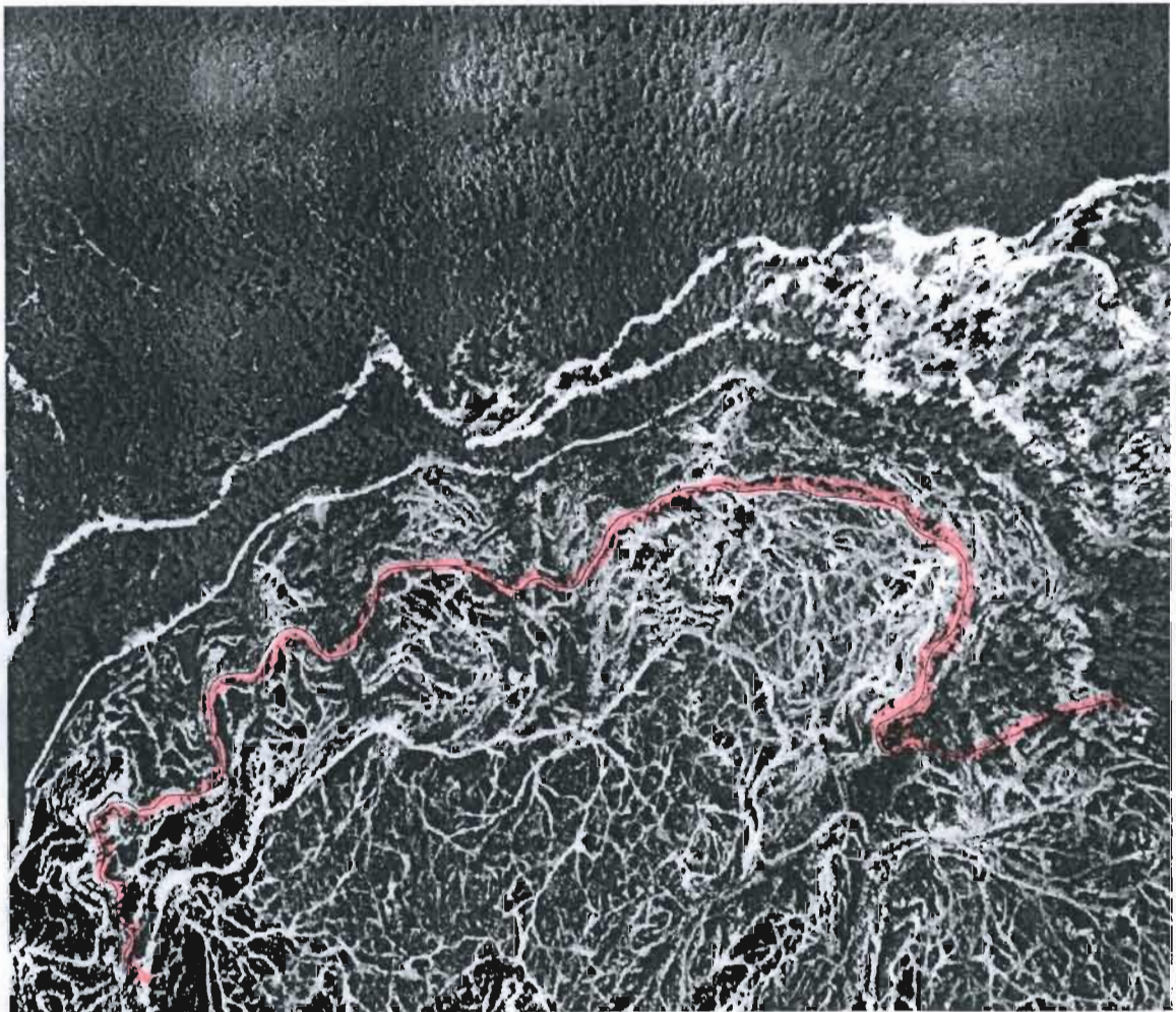
FIGURE 4. AERIAL PHOTOGRAPH SHOWING EXTENT OF LOGGING AND RELATED ROAD CONSTRUCTION BY 1974 NEAR THE L-2-2-1. ALL WHITE LINES ARE EITHER HAUL ROADS OR SKID TRAILS. THE L-2-2-1 ROAD IS HIGHLIGHTED IN ITS ENTIRETY. OLD GROWTH REDWOOD FOREST OCCUPIES THE UPPER THIRD OF THE PHOTOGRAPH, WHERE INDIVIDUAL TREES AND THEIR SHADOWS ARE VISIBLE.
