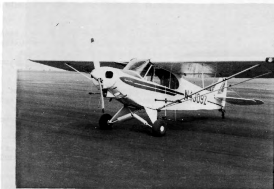
Fig. 4 Piper Supercub ready for radio-tracking. Stacked Yagi antennas are attached to wing struts. The rotatable Yagi antenna can be seen behind the left front wheel.
