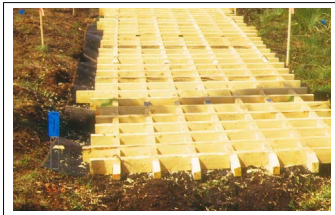
Figure F. Wood Matrix material tested for ATV trail mitigation in Wrangell-St. Elias National Park and Preserve.
