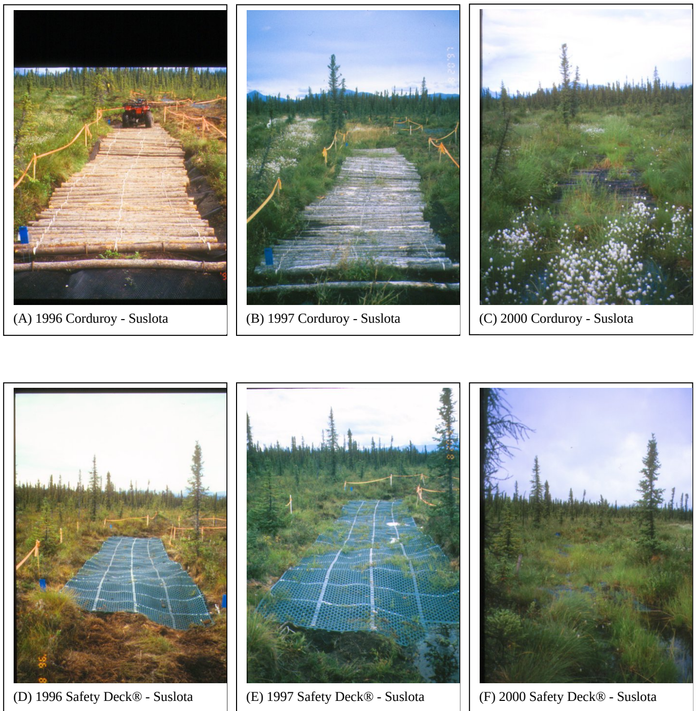
Figure 21. Photo series of Corduroy (A-C) and Safety Deck (D-F) hardening material plots between 1996 and 2000 at Suslota Lake study site in Nabesna District, Wrangell-St. Elias National Park and Preserve, Alaska. This study site had ATV use during 1996 and 1997; an alternative trail was developed in 1998 that by-passed the study plots.
