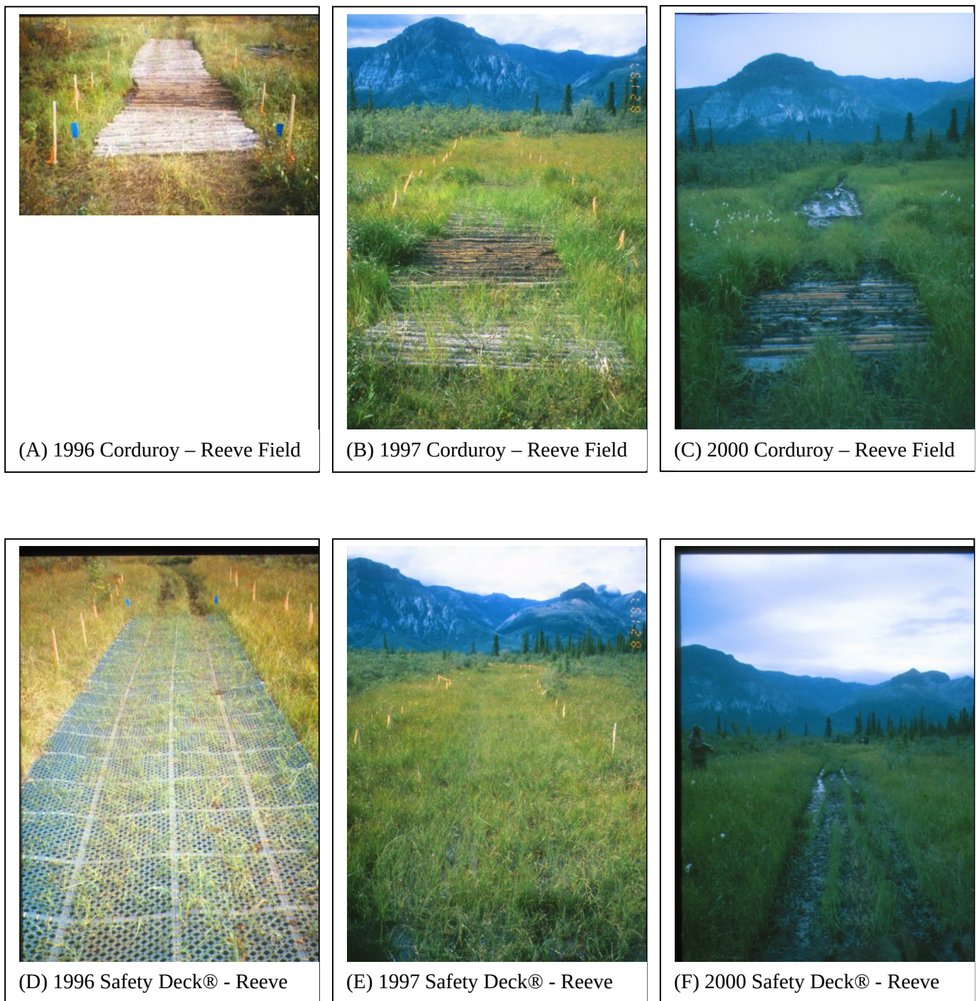
Figure 17. Photo series of Corduroy (A-C) and Safety Deck (D-F) hardening material plots between 1996 and 2000 at Reeve Field study site in Nabesna District, Wrangell-St. Elias National Park and Preserve, Alaska.
