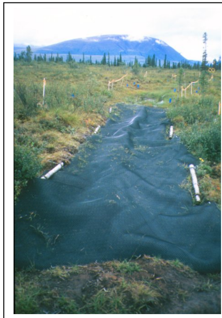
Figure D. Polynet PN-3000/Pyramat™ tested for ATV trail mitigation in Wrangell-St. Elias National Park and Preserve
