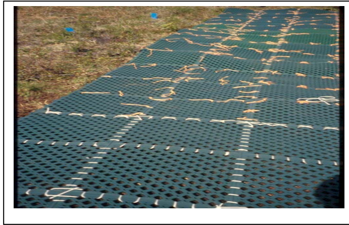
Figure E. Safety Deck® material tested for ATV trail mitigation in Wrangell-St. Elias National Park and Preserve.
