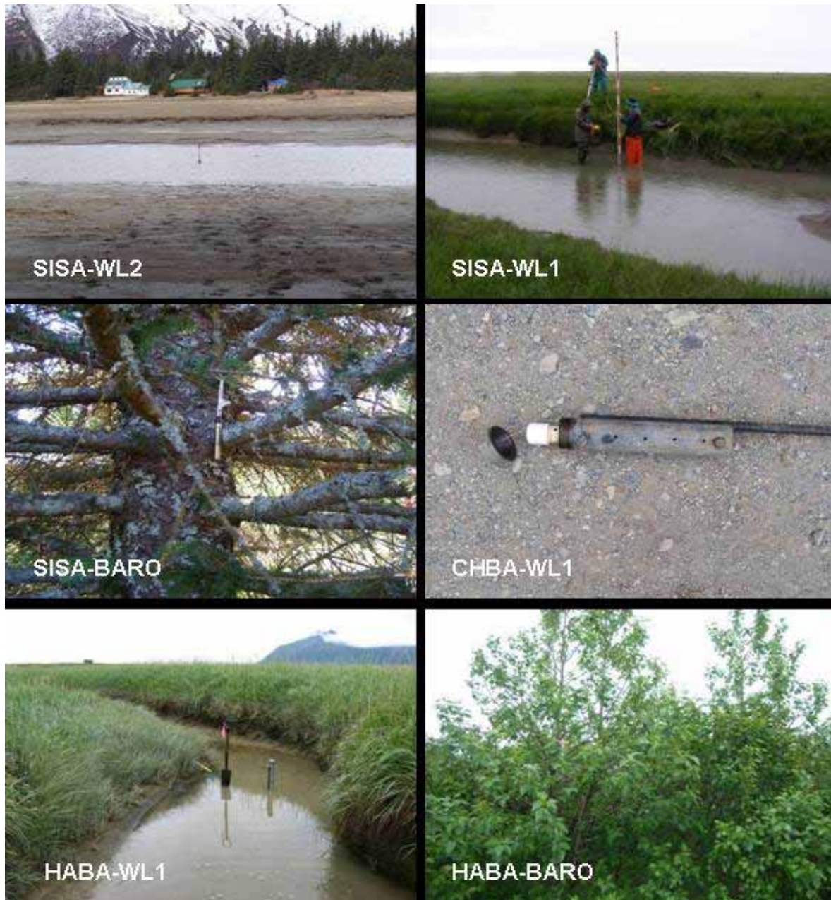
Figure 11. Views of water level and barometric pressure recorders at the Silver Salmon (SISA), Chinitna Bay (CHBA), and Hallo Bay (HABA) coastal sites.
