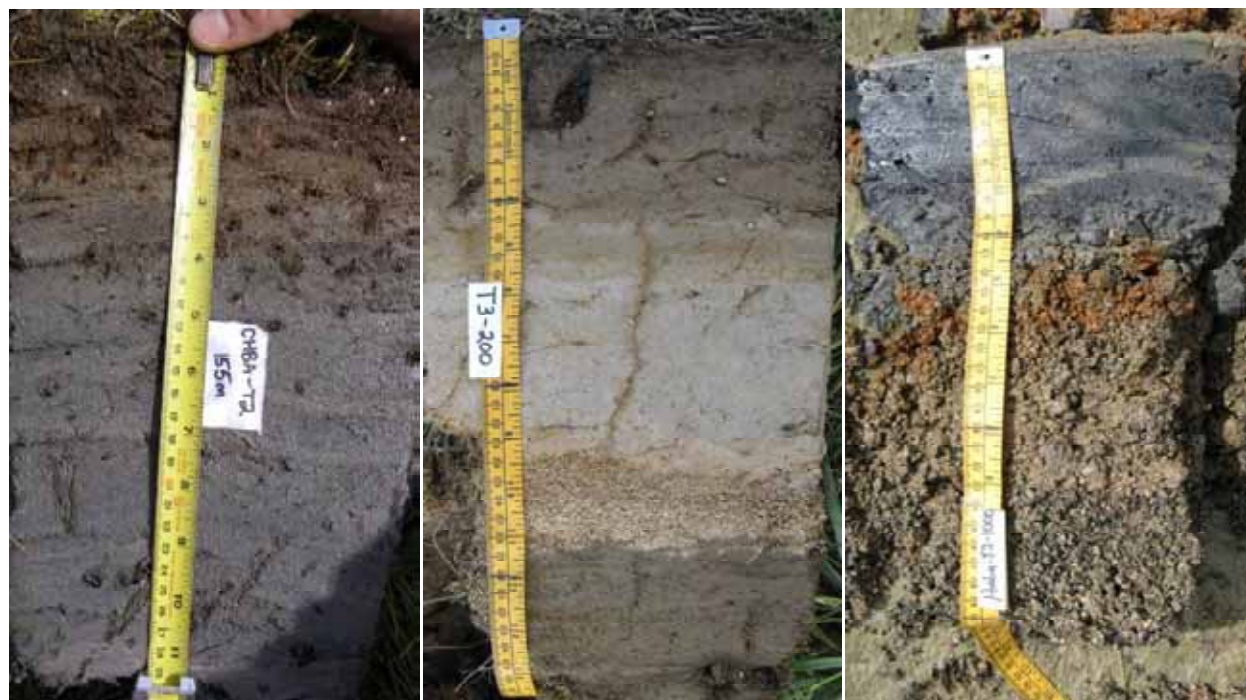
Figure 14. Photographs of soil plugs extracted for documenting current sediment layers and stratigraphy for use in future measurement of sediment accumulation.
