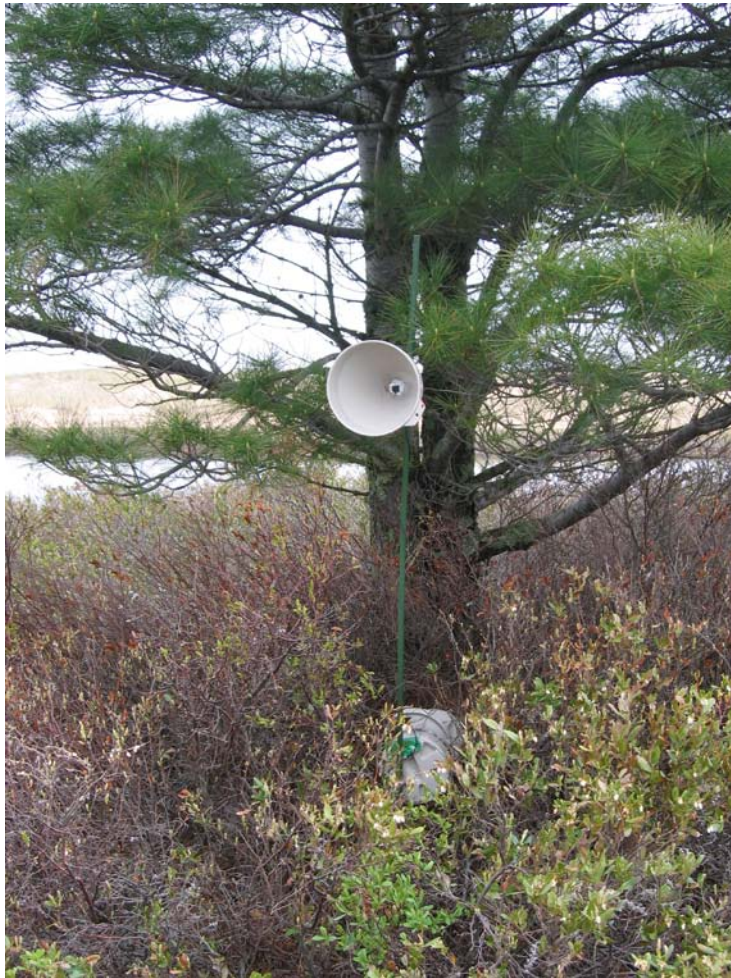
Figure 10. The Diasonic Voice Bank remote call recorder (Diasonic Co. Ltd., Anyang City, South Korea) at Stockton Island Lagoon, Apostle Islands National Lakeshore, Wisconsin. This unit was placed on-site on 25 May 2006.
