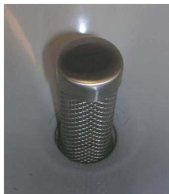
Figure B8. Assembly filter.
