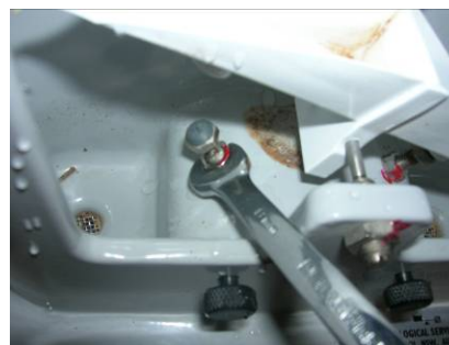
Figure B6. Loosening locknut.
