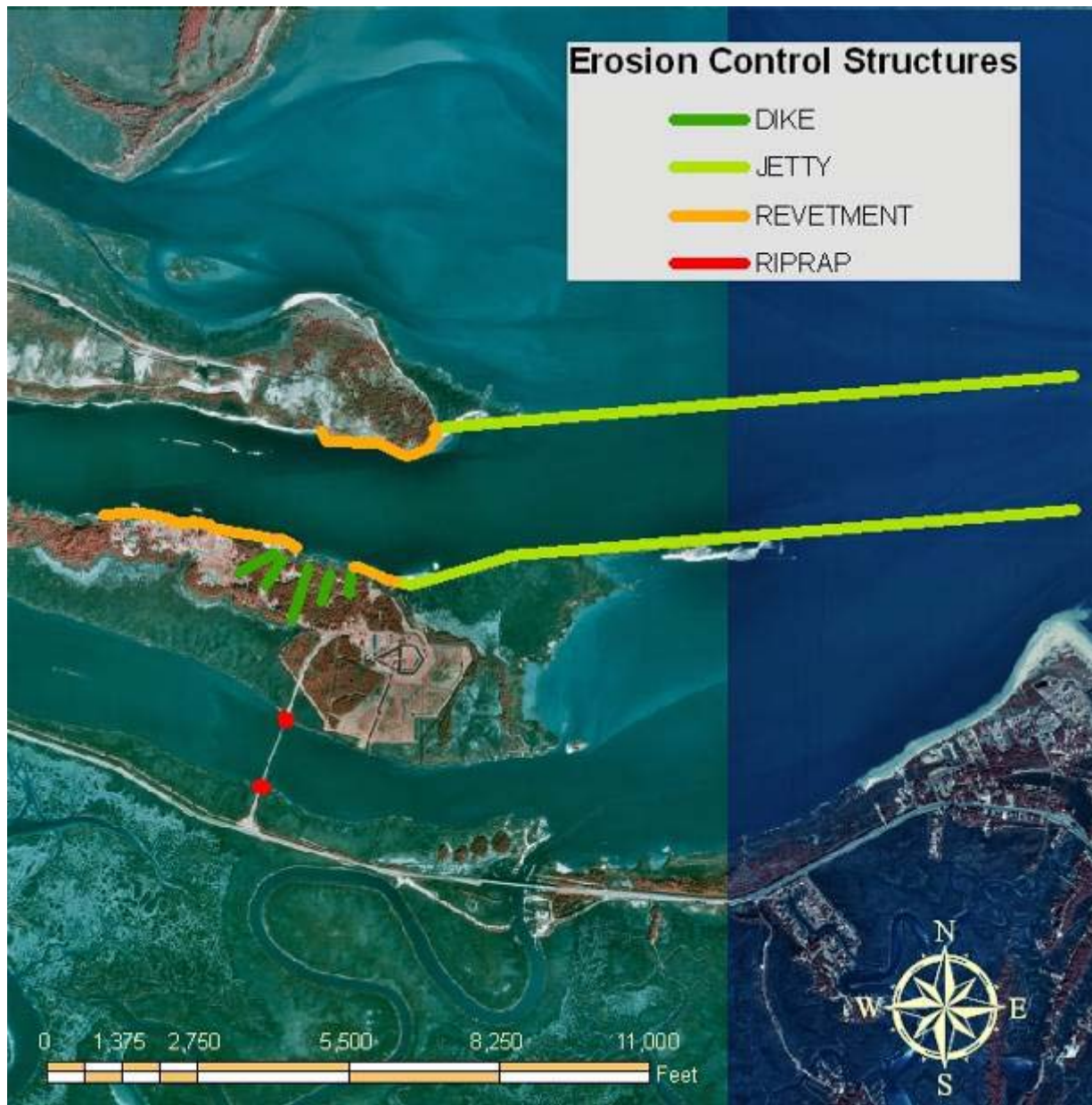
Figure 41. Erosion control structures in FOPU.
