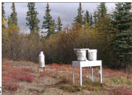
NADP site in Denali NPP includes a wet deposition collector and electronic rain gage. A similar system will be installed in King Salmon in spring 2009.
