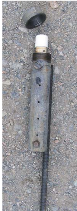
Figure 5-1. Metal pipe and rebar housing for water-level datalogger.
