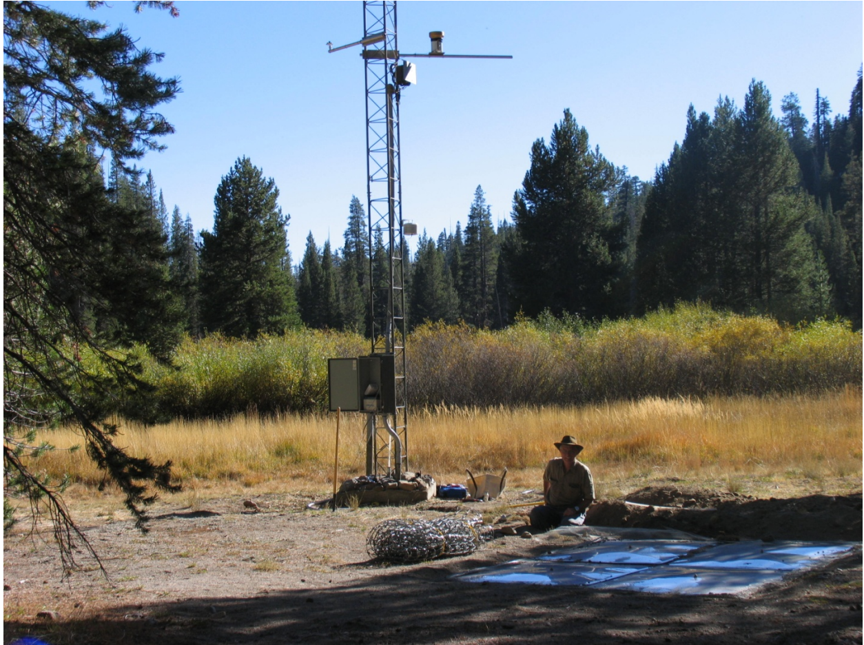
Figure C-5. Frank Gehrke putting the final touches on the snow pillows at the Soda Springs weather Station, Devils Postpile NM. Note the minimal amount of instrumentation on the tower. 28 September 2008.
