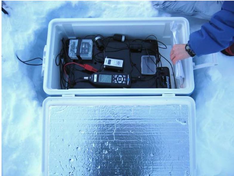
Sound monitoring equipment placed inside a cooler for protection against cold temperatures
