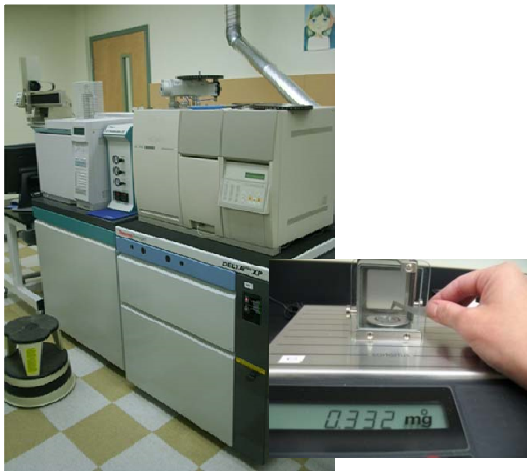
Loading samples in tin cups (right) and measuring for stable isotope analysis using the Isotope Ratio Mass Spectrometer (left) (Photos courtesy of ASLC and ASIF 2008)
