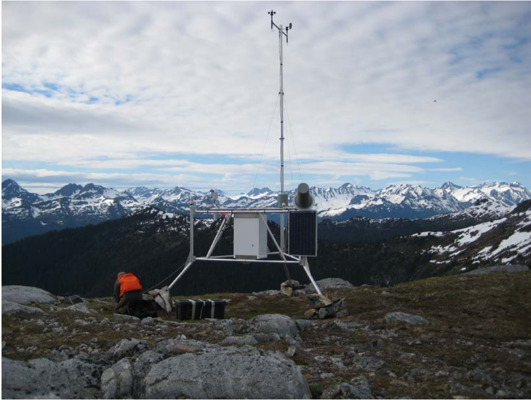
Note the rocks anchoring the feet of the RAWS. 7-2-08
