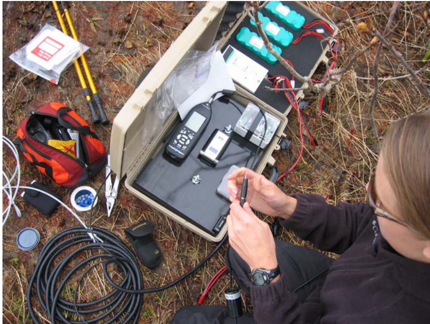
Acoustic Technician checking the battery voltage levels at a monitoring site.
