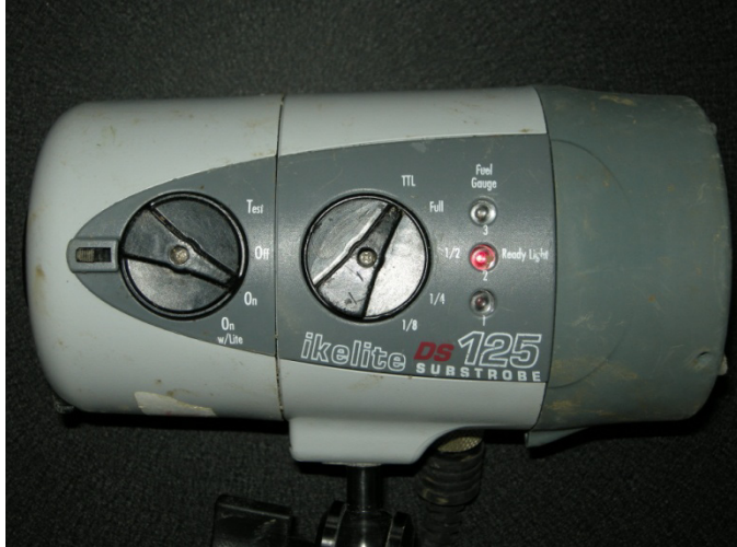
Figure 23. Strobe settings during photography for the DS-125 strobe. The “Ready Light” should illuminate. The DS-160 strobe uses the same settings.
