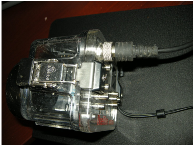
Figure 26. Photograph showing the connection location of the strobe to the camera.
