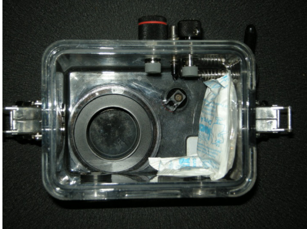
Figure 25. Front of camera housing showing correct placement of the moisture muncher. The housing for the Nikon Coolpix is shown, but the moisture muncher should be in the same location in the Canon PowerShot housing.
