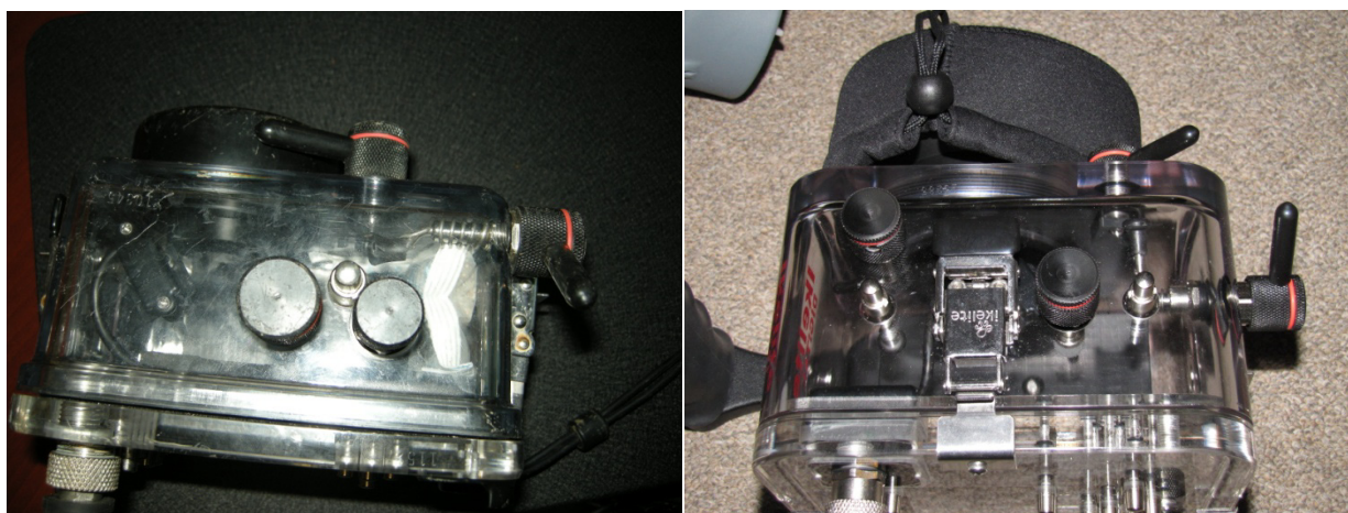
Figure 22. Top of the Ikelite camera housing (left, Nikon Coolpix; right, Canon PowerShot). The command dial is the large black knob on the right for the Nikon Coolpix. The command dial is the black knob on the left for the Nikon Coolpix. The mode dial is the left knob on the Nikon Coolpix and the right knob on the Canon PowerShot.
