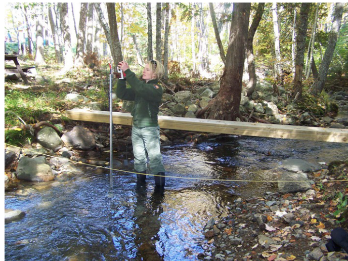
Figure 3. Meghan Goff obtains a discharge (streamflow) measurement with a Price pygmy current meter. (Photo by B. Arsenault)
