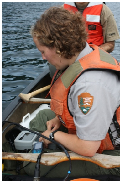
Figure 2. Beth Arsenault takes a lakewater chemistry profile with the YSI multiparameter sonde. (Photo by M. Goff)
