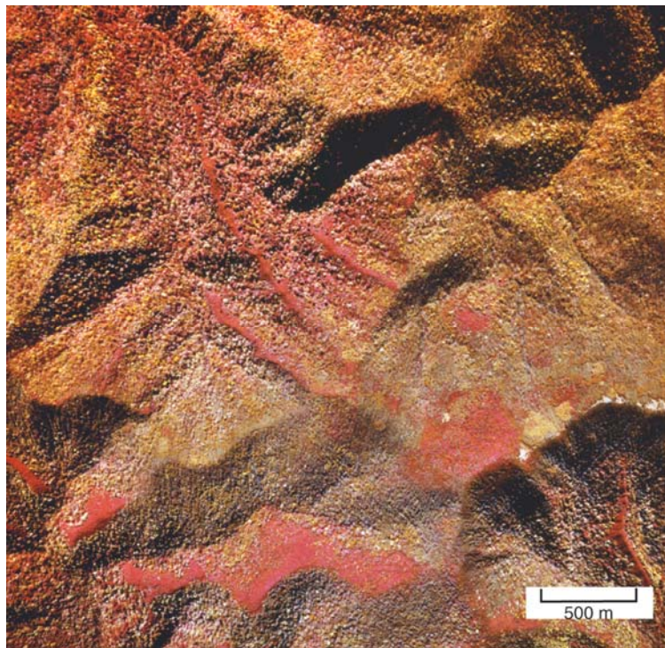
Figure 3. An example of a large-scale color infrared aerial photograph recorded in October 1997 and used for photo interpretation of vegetation detail.
