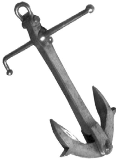
Figure 18. Porter's style bower anchor, similar to the Austria's (Curryer, 1999, p. 77).
