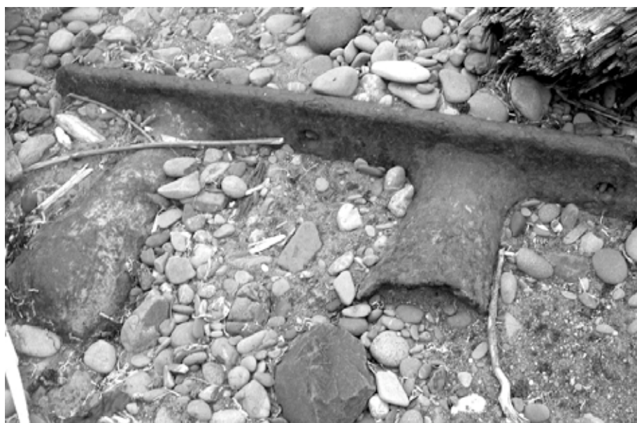
Figure 28. A set of double bitts from the Austria .
