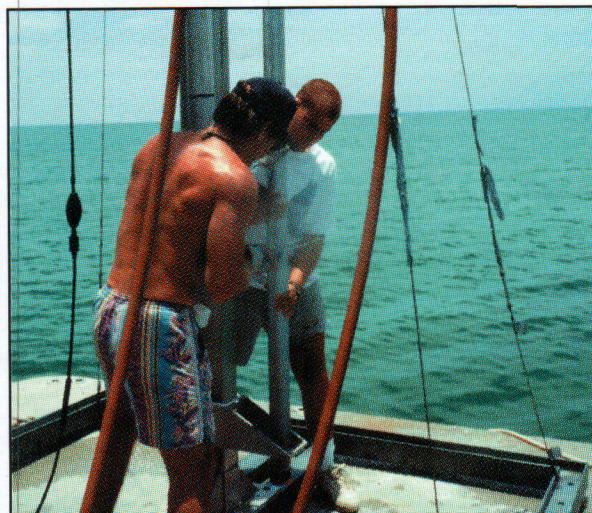
Researchers take vibracore samples to examine sediments lying below the sea floor.
