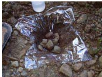
Figure 2. Hole with plastic wrap and stones used to determine soil bulk density.
