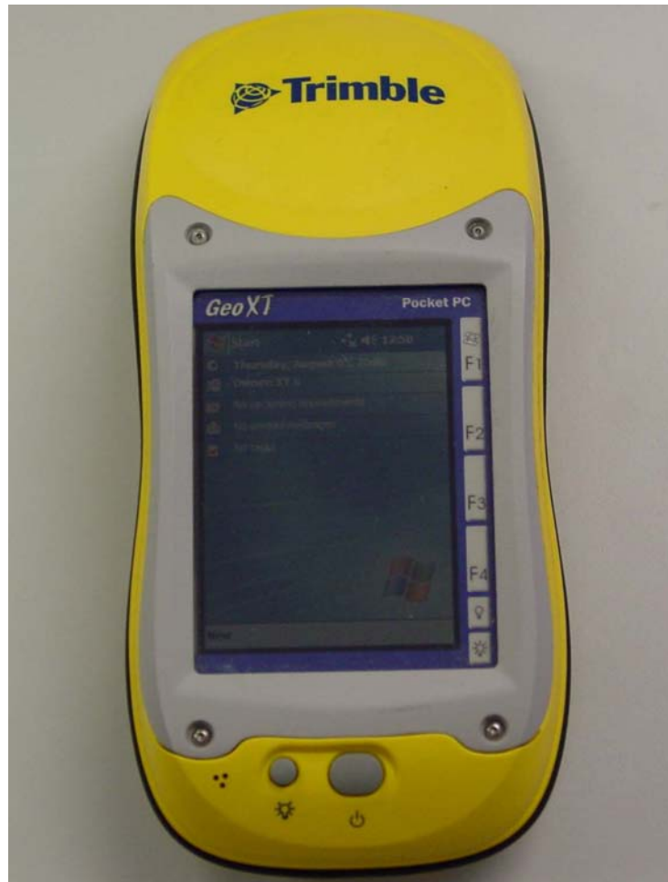
Figure 1.1. Trimble GeoXT GPS unit
