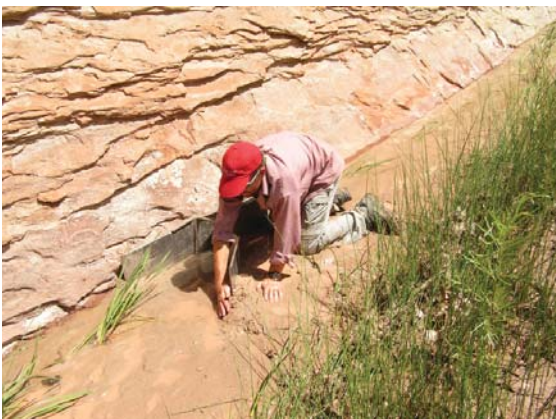
Measuring discharge at Lower Echo Canyon Spring, Colorado National Monument.
