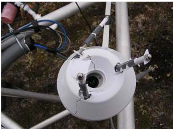
Figure 6. AT-RH sensor was destroyed (Contact Creek RAWS).
