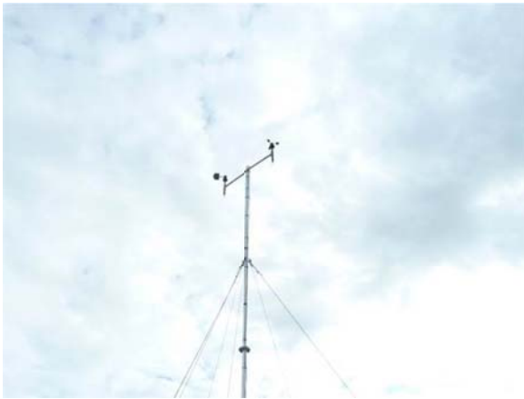
Figure 13. The tail (fletching) had broken off the wind direction sensor (Fourpeaked RAWS).
