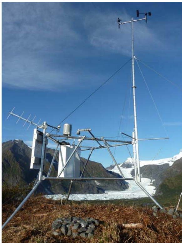
Figure 42. Photograph of the station and Pedersen Glacier after maintenance was completed (Pedersen Lagoon RAWS). Barbed wire was added to the top of the tri-leg tower in order to protect sensor cables from damage by wildlife.
