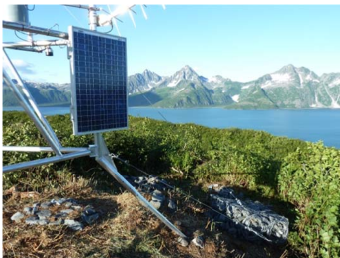
Figure 33. Guy lines from the station and mast attached to a 1500 lb gabion (Pedersen Lagoon RAWS).
