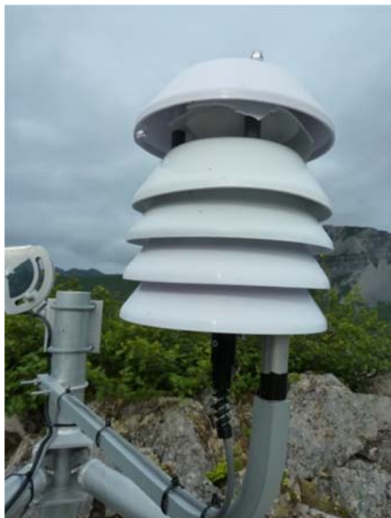
Figure 17. Damage to the AT-RH sensor shielding (Hickerson Lake RAWS).
