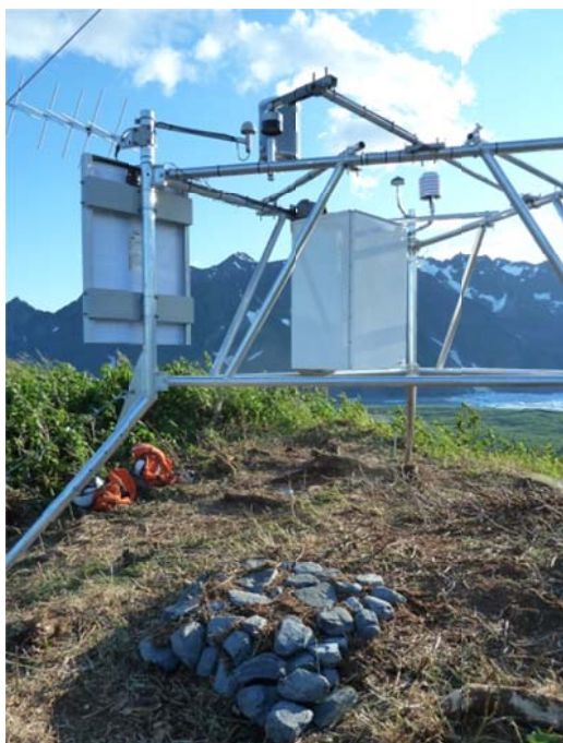
Figure 35. Snow depth sensor (sonic distance ranger) and reflector surface constructed of beach rock and soil (Pedersen Lagoon RAWS).
