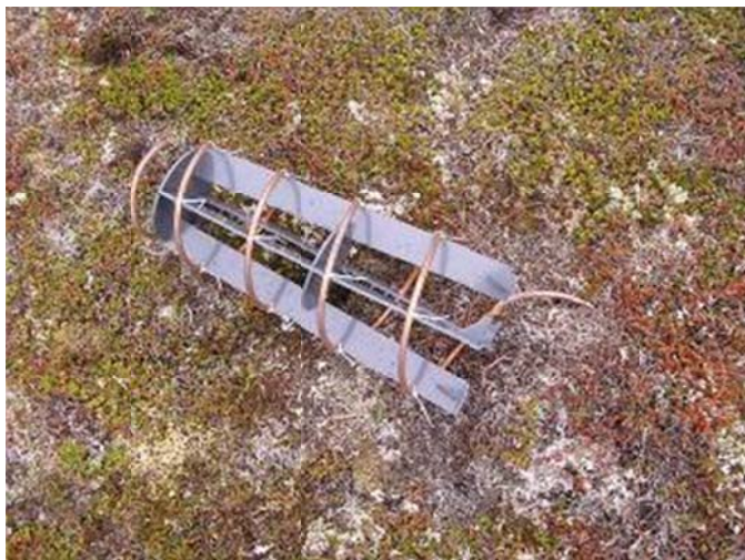
Figure 5. GOES antenna was destroyed and lying on the ground (Contact Creek RAWS).
