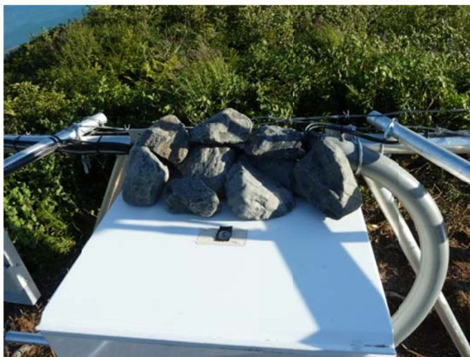
Figure 37. Rocks were piled on top of the instrument enclosure to help mitigate damage from wildlife (Pedersen Lagoon RAWS).
