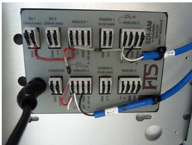
Figure 47. Configuration of the analog input module for the soil temperature sensors (Snipe Lake RAWS).
