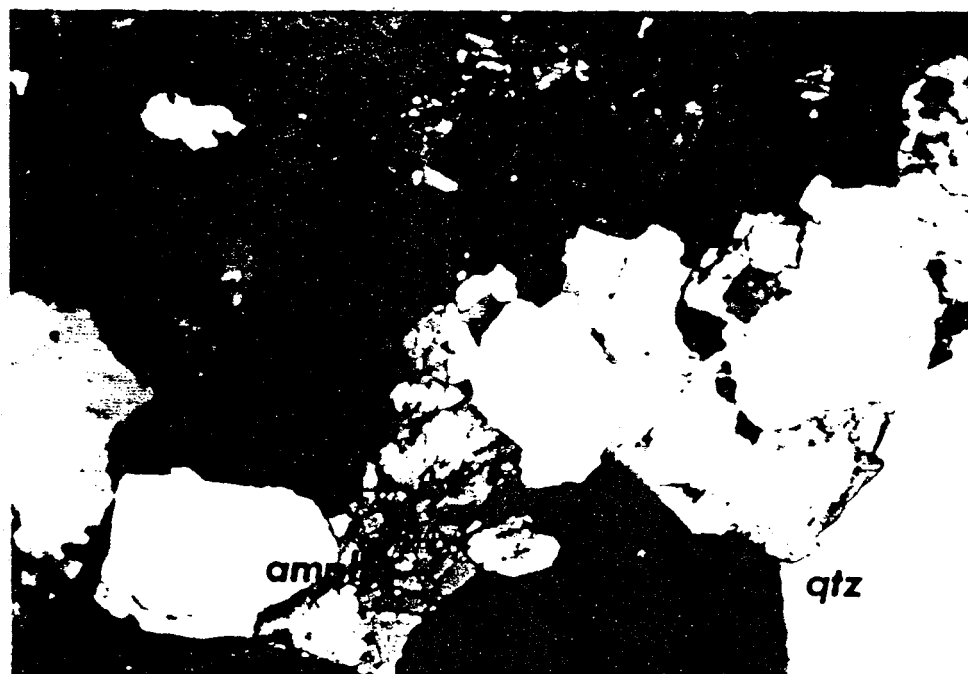
PLATE 3-15: Granitic unit, FJV-6, with amphibole crystal. Crossed polars. Field of view=3mm. 'C' on stratigraphic column (Figure 2-2).
