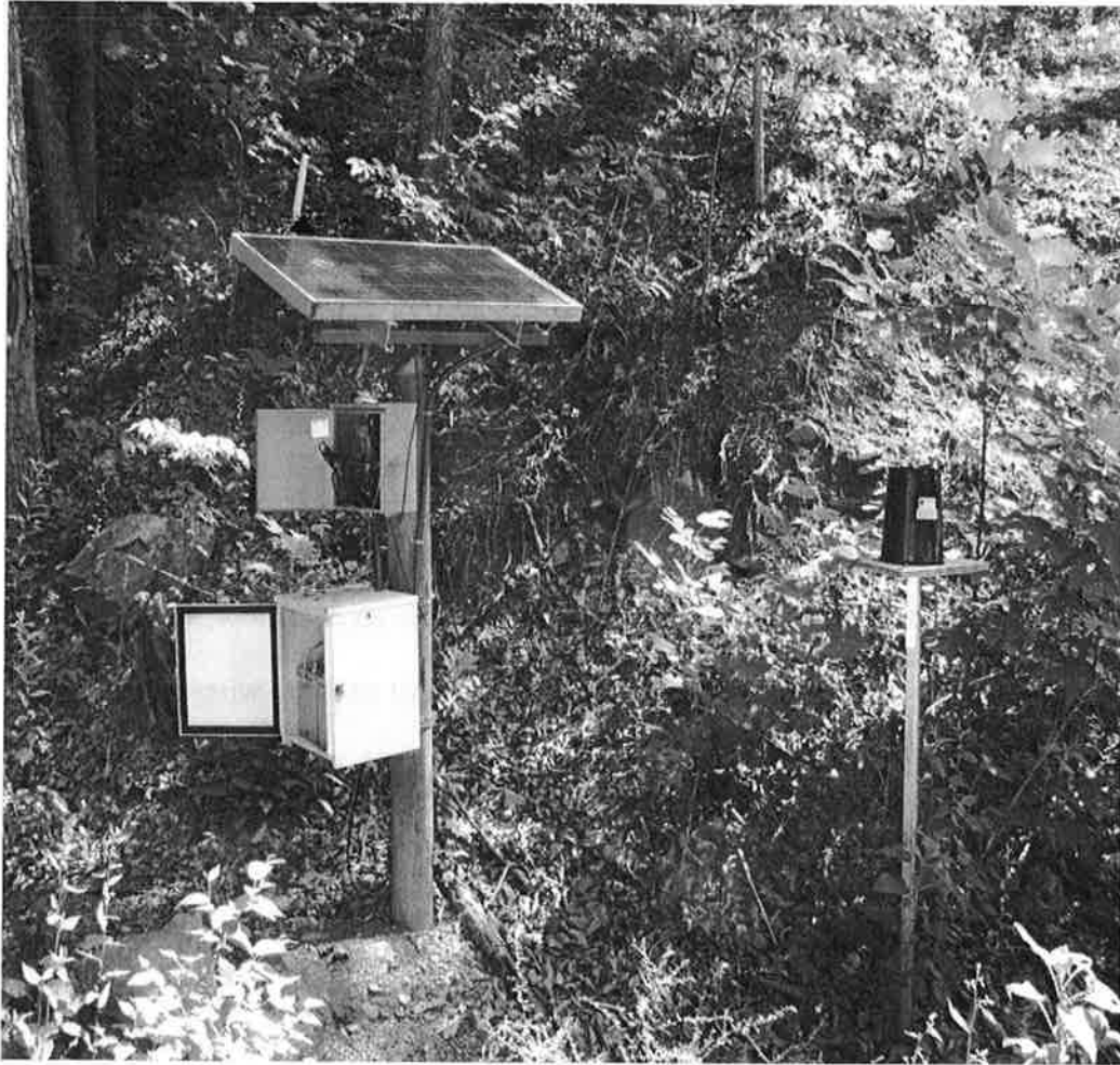
Figure 3.9: Station setup at HH showing solar panel, equipment boxes, and rain gauge.
