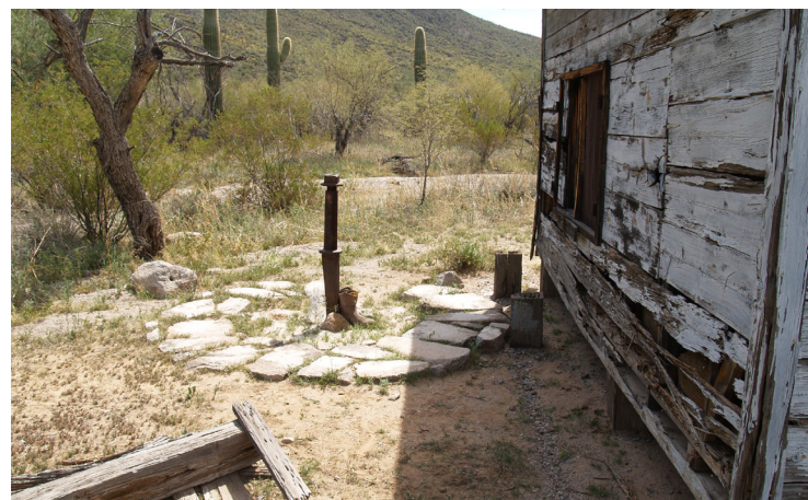
Figure 9: The Arrastra, a device for milling ore, is located immediately adjacent to the Bunkhouse. Because it would have been impossible to use the arrastra as it is currently located, it is assumed that it was in place prior to the placement of the bunkhouse, and was no longer in use at that time.
