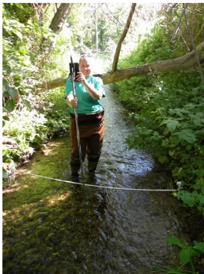
Figure 19. Technician setting tagline and stream section with automated AquaCalc Pro and pygmy meter setup.
