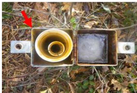
Figure 23. Stainless steel well casing as benchmark for pond stage measurements.
