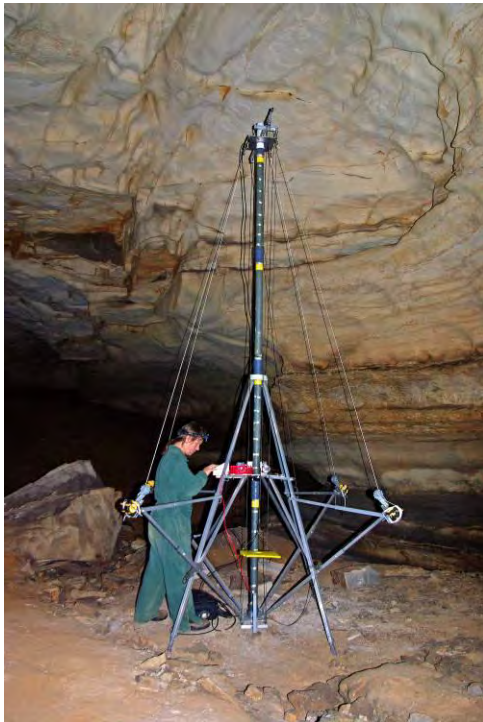
Figure 22 – Photo of instrument lift system. Air temperature and relative humidity sensors are attached to the tower, one at the top of the tower and one on the back-left leg of the tower base. NPS photo by Kurt Helf.
