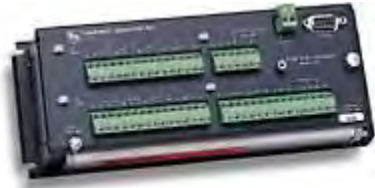
Figure 3 – Campbell Scientific's CR10X Datalogger for Measurement and Control. Image downloaded from www.campbellsci.com .
