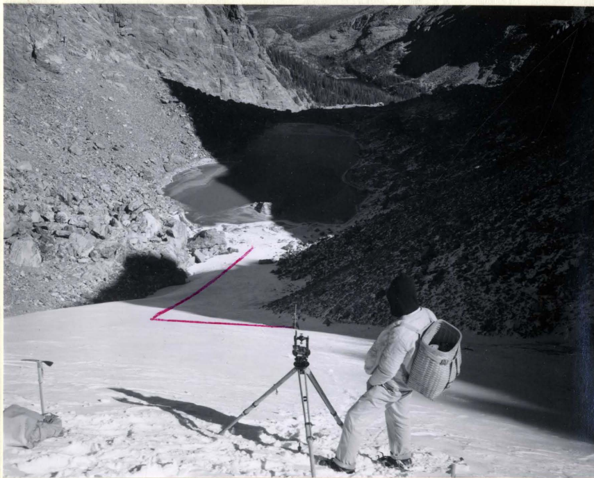
Longitudinal Traverse on Andrews Glacier Red line represents offset of survey at lower end of glacier. (See survey statistics)
