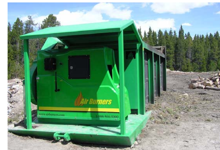
Figure 21. An Air Burner is used to burn infected wood being removed from RMNP. Due to air quality issues from traffic and even China, RMNP is using this firebox to reduce emissions. Photo: Amanda Jeter (2008)
