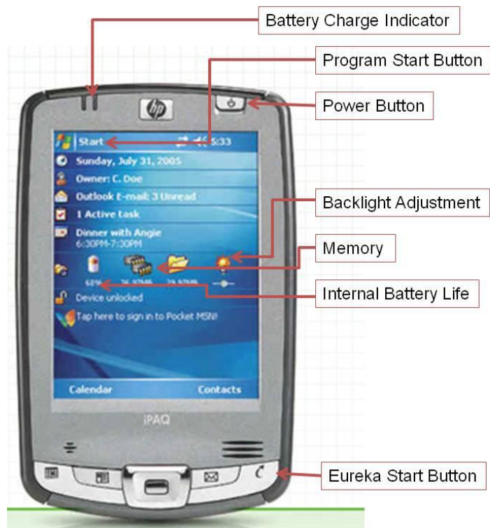
Figure 17. Hewlett-Packard iPAQ overview, showing relevant buttons to Manta multiprobe function.
