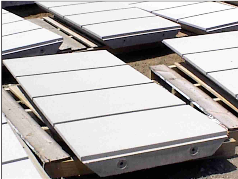
Typical Pilaster Covers
