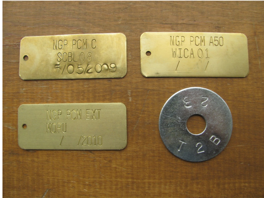
Figure 6. A sample of tags and washers used to mark long-term vegetation monitoring plots in the NGPN. From the top left and working clockwise: a center tag from PCM-08 in SCBL evaluated on May 5, 2009; a tag used to mark the end of the A transect at WICA PCM-01; a tag used to mark the center of an extensive plot in MORU; and a washer used to mark the beginning of the second tree transect. In all cases, the tags are close or flush to the ground. The brass tags are fixed to rebar with wire, and the washer is held in place by a large nail.
