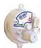
Figure 16. Onset Computer Corporation’s HOBO Pro RH/Temp Datalogger. Image downloaded from www.onsetcomp.com .
