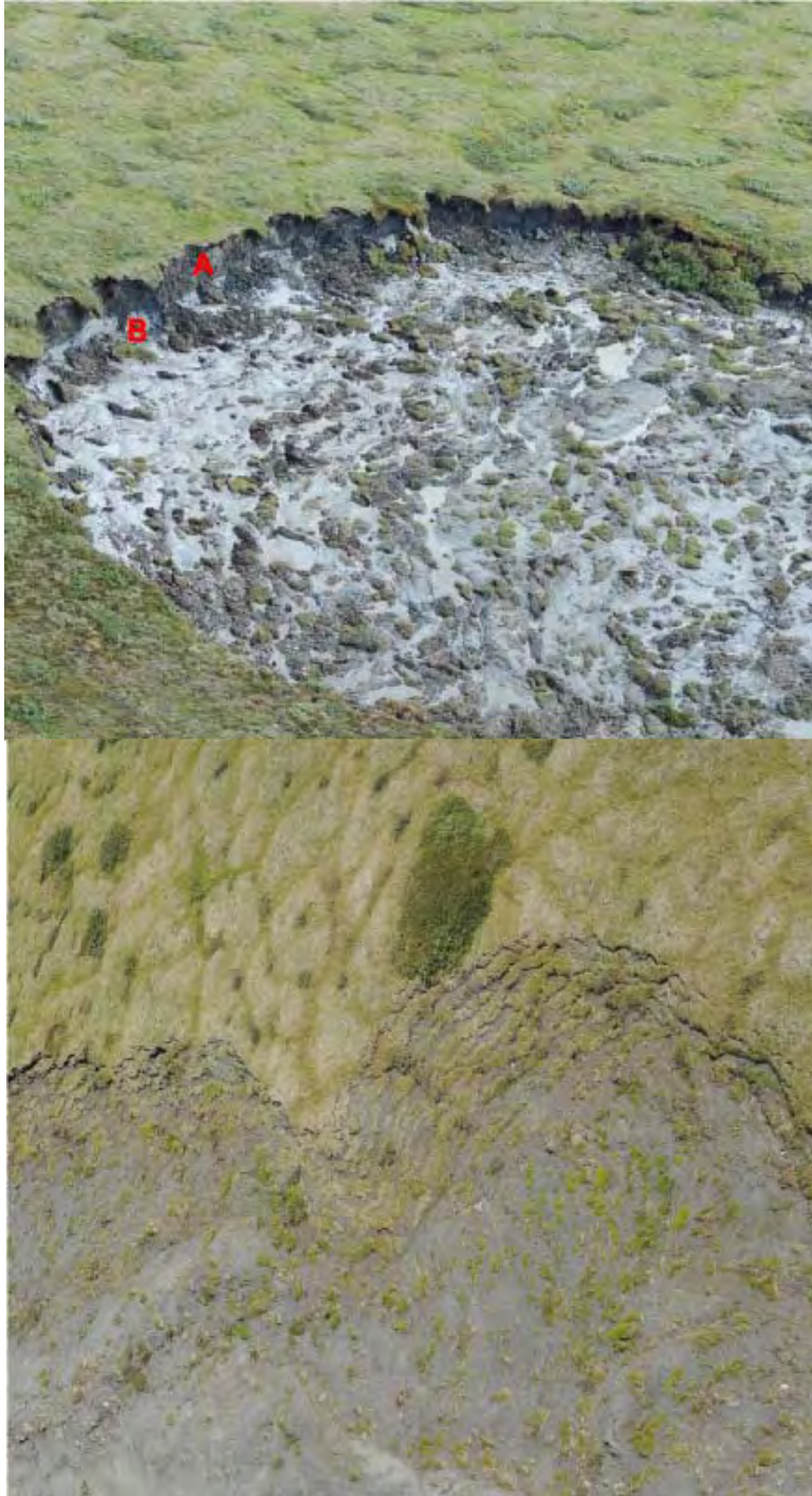
Figure 29. Oblique aerial photographs of the main scarp of slump NOAT161 in 2011. The southeast portion (upper photo) was nearly vertical with glacial till (A) over glacial ice (B). Most of the rest of the main scarp (lower photo) was sloping with extensional flow resulting in numerous parallel cracks in the vegetation mat.
