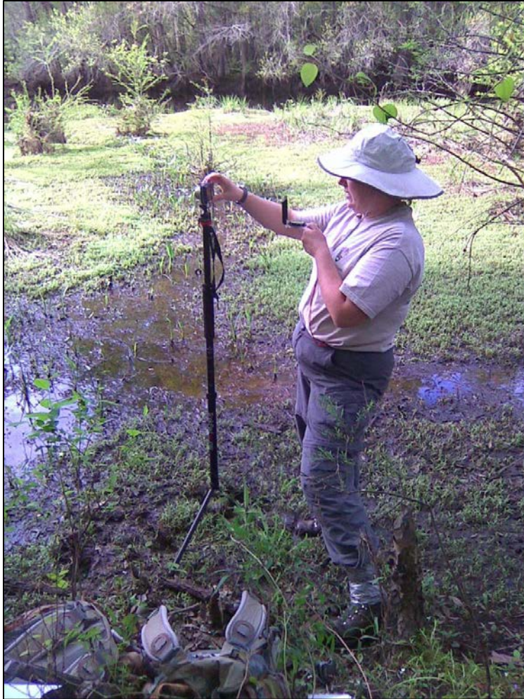
Figure 1. Example of the tripod setup and identification of the cardinal directions with a compass.
