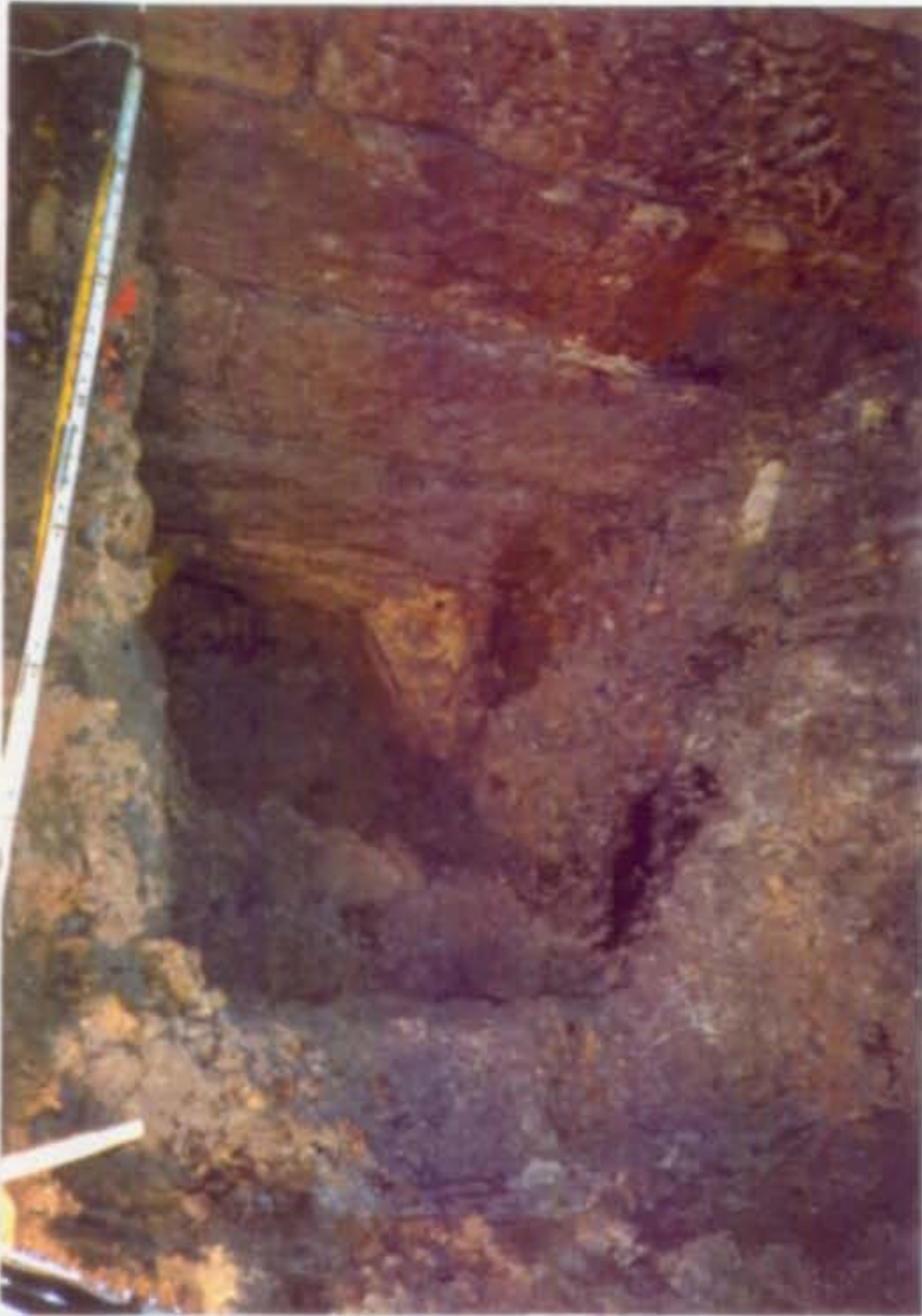
Test Pit No. 1: Sandstone bedrock foundation for west masonry lining at Sta. 0+59.
