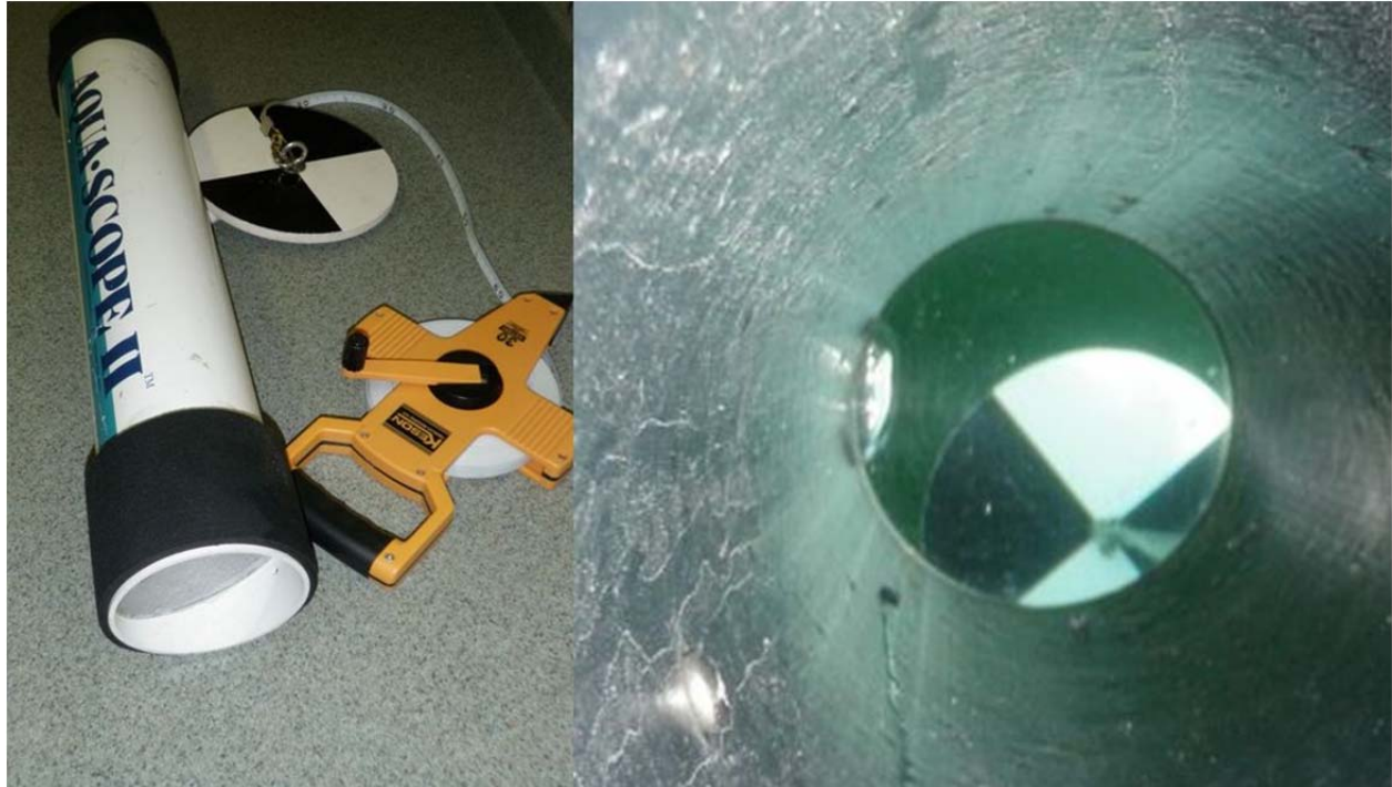
Figure 9. Secchi disk, measuring tape, and viewing scope (left) and view of submerged Secchi disk through viewing scope (right).
