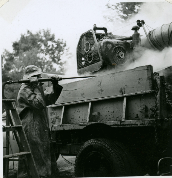
Cleaning Oliver Mist Sprayer with steam hose after use in insect spraying program in Acadia National Park.
