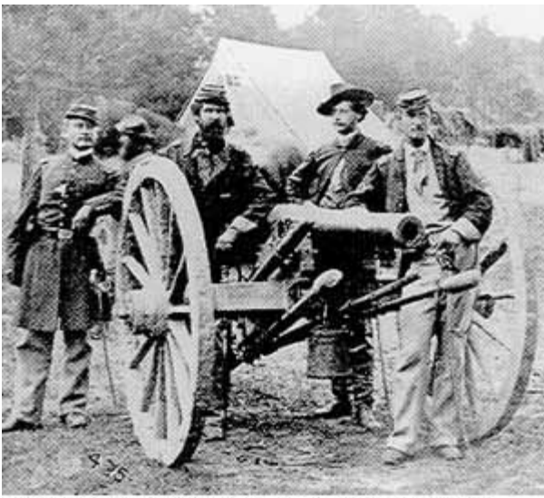
Figure 55 - Union officers of the Second U.S. Artillery were photographed circa 1863 with a 3-inch Ordnance Rifle. The weapon weighed about 850 pounds, with a bore 3.67 inches in diameter. The Ordnance Rifle, mounted on an oak carriage, had an effective range of about 3,500 yards and required a standard crew of 11 men. Each gun, drawn by four horses, was attached to a limber with one limber chest. The gun was supported by a caisson drawn by the limber or occasionally by four horses. The caisson had two additional limber chests. The artillery section at Monroe's Crossroads was two 3-inch Ordnance Rifles. A Section could be supported by one battery wagon and/or a forge wagon, each drawn by four horses. The limber chest contained rounds of 25 fixed shot, 20 case shot, and five canister.
