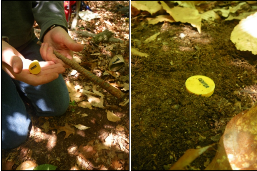
Figure 3. Example of rebar and center cap.
