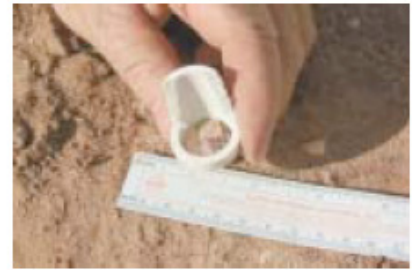
Figure 8-5. Ensure correct sample size
