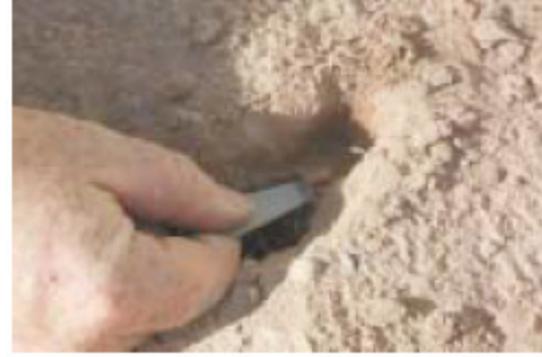
Figure 8-7. Collect subsurface sample
