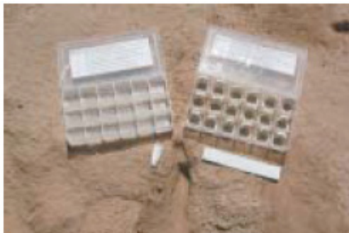
Figure 8-8. Complete soil stability kit with water and samples
