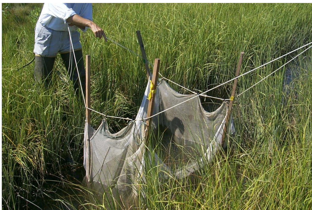
Figure 4. Photo of ditch net deployed in a ditch with doors down (top photo) and with doors up (bottom photo) (photos courtesy of M. J. James-Pirri).
